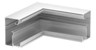
Internal corner base to create a design device installation trunking of the GAD series. 45 mm system opening for acceptance of Modul 45 switch and connection devices and the appropriate PVC and aluminium covers of the Rapid 45 series. The fitting can be completed with fitting covers in the "Swing", "Soft" or "Style" design. The GAD OTA cover adapters are essential. GAD OTD spacer must be placed between the trunking covers.
