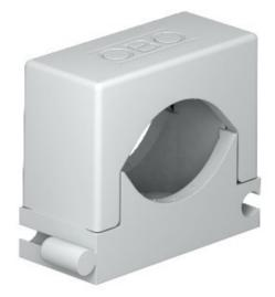
Universal clip for the single fastening of cables and pipes, all sizes can be seamlessly expanded among each other, with adhesive foot, slot and for screwing to M6 thread. To stick the polyamide clips to masonry and concrete, use the Impu-Fix ribbon conductor quick adhesive, type 509.
