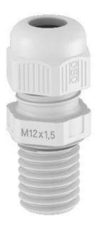
The quickest and most convenient way of providing strain relief and tightness with cable glands on junction boxes and housings is with the tried-and-trusted V-TEC VM cable glands from OBO. With the integrated sealing lip and the special OBO lamella technology protection class IP68 is achieved. Strain relief and tightness have been tested to DIN en 50262.
