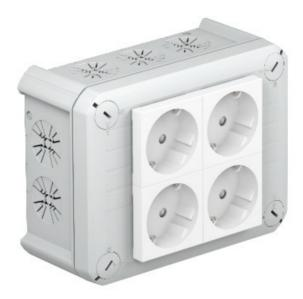
The junction boxes are made of a thermoplastic polypropylene polymer and are equipped with strain relief entries. These entries can be penetrated directly with the cables. The special structure of the opening means that the cables cannot be removed unintentionally. Suitable for cable diameters of between 7 and 21 mm Depending on the type, the cover contains two or four Modul 45 protective contact sockets in red or white.
