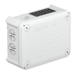
All the T series junction boxes are UV-resistant. They are made of polypropylene (thermoplastic polymer) and are equipped with strain relief entries and preterminated Wieland connection sockets, type GST-18-i3 (s = black, w = white, r = red). The strain relief entries can be penetrated directly with the cables. The special structure of the opening means that the cables cannot be removed unintentionally. Suitable for cable diameters of between 7 and 21 mm
