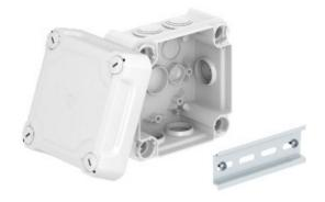
The junction boxes consist of thermoplastic material. The bottom parts are made from impact-resistant polypropylene, the box cover is made from extremely hard-wearing, impact-resistant polycarbonate. The high IK 10 impact resistance at -5°C shows this also.
