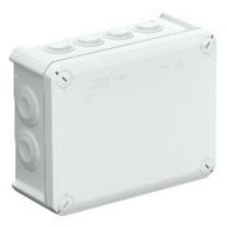
The junction boxes are made of a thermoplastic polypropylene polymer with plug-in seals made of ethylene vinyl acetate (EVA). This allows installation of cables either directly through the 7x M25 + 5x M32 seals, or the seals can be cut with a knife at the pre-marked points, in order to create an insertion opening for cables or pipes. Alternatively, cable glands can be pushed through the openings instead of the seals and locked with a locknut from the inside.
