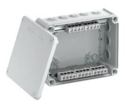
All the T series junction boxes are UV-resistant. They are made of a thermoplastic polypropylene plastic with plug-in seals made of ethylene vinyl acetate (EVA). This plastic is soft, which means that it is malleable. This allows installation of cables through the 9x M25 + 7x M32 seals, or the seals can be cut with a knife at the premarked points, in order to create an insertion opening for cables or pipes.
