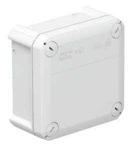
The junction boxes are made of a thermoplastic polypropylene polymer with closed side walls. This means that the required openings can be made wherever they are required. EDK plug-in seals or cable glands with locknuts can be inserted in these openings, to allow cable insertion.
