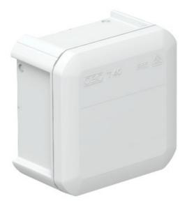
All the T series junction boxes are UV-resistant. They are made from polypropylene (a thermoplastic material) and have closed side walls. This means that the required openings can be made wherever they are required. EDK plug-in seals or cable glands with locknuts can be inserted in these openings, to allow cable insertion. The junction boxes can be mounted on mounting plates in the openings on the floor
