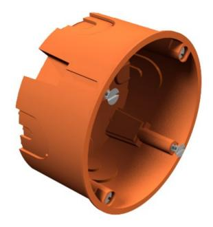
Cavity wall accessory socket. Dimensions to DIN 49073-1, for plate thickness 7-35 mm Standard combination spacing 71 mm, option for continuous wiring using connection support for combinations between accessory sockets and accessory connection sockets, 8 break-out openings for NYM cables, data cables and pipes Ø 20 mm, accessory sockets can also be used as connection sockets to VDE 0606-1 with double bolt fastening and screw-on cover, protection rating IP20.
