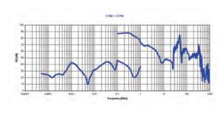
Shielding effectiveness for top and bottom plates of the MultiFlex range
