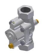
Cooling water regulating valves of type WVTS are suitable for controlling the temperature of a flow of water or neutral brine. WVTS water reg. valve opens on rising sensor temperature. Large self-acting cooling water regulating valves for accurate flow control based on sensor temperature Open on rising temperature Cast iron valve body Thermostatic pilot elements (2 or 5 m capillary tube) ordered separately
