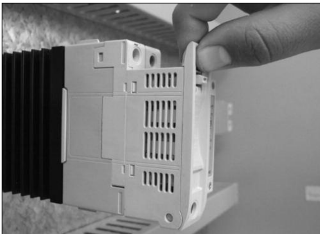
1. Preparation for opening fuse holder.
