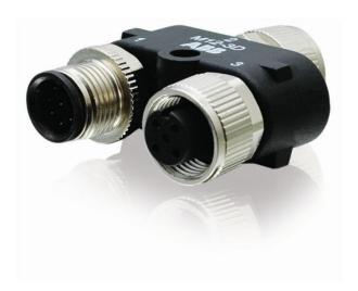
M12 Y connector for series connection of dynamic safety devices such as Eden Sensors, Smile E-Stops, Inca E-Stops, Spot Single Beams, and Tina Dynamic Adapters. 5-pole M12 female connector(2) for connection of the safety device, 5-pole M12 male connector(1) for connecting 24VDC, 0VDC and the dynamic transmit signal to the field devices and 5-pole M12 female connector(3) for either the continuation of the circuit or the return of the dynamic receive signal to the Vital 1/Pluto controller.
