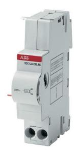
The S2C-UA 230 AC undervoltage release has the function to protect the load in case of a voltage drop included between 70% and 35% of its rated value. Positive safety (device tripping when the voltage is disconnected) emergency stop by means of a button. Suitable for MCBs S200 series, RCCBs F200 series and RCBOs DS201, DS202C, DS200 series. It can be used with MCBs SN201 series by means of SN201-IH interface module. Rated voltage: 230V a.c.
