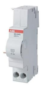
The S2C-OVP1 overvoltage release has the function of monitoring voltage between the neutral and phasewhen an overvoltage reaches the threshold value, the OVP causes the tripping of the associated device. Suitable for S200 MCBs up to 63A, F200 RCDs up to 100A and DS201-DS202C RCBOs. Max tripping voltage: 275V a.c.
