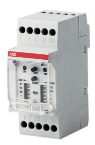
Residual current monitors (RCMs) with external transformer can detect leakage currents. Through minidip you can set sensitivity and intervention time. Operating voltage: 230...400V a.c.
