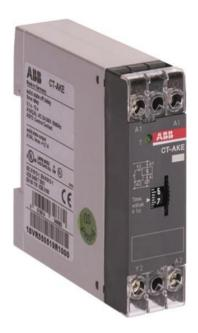
The CT-AKE is a single-function electronic time relay from the CT-E timer range. It provides an OFF-delay (delay on break) function with a time range from 0.1 s to 10 s. This time relay operates with a rated control supply voltage of 24 - 240 V AC / DC and has a solid-state output.
