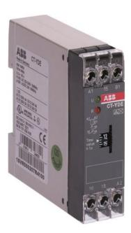
The CT-YDE is a single-function electronic time relay from the CT-E timer range. It provides a star-delta function with a time range from 0.3 s to 30 s. This time relay operates with a rated control supply voltage of 24 V AC / DC / 220 - 240 V AC and has a 1 c/o (SPDT) output rated at 250 V / 4 A.
