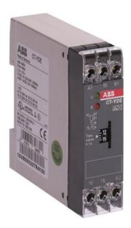
The CT-YDE is a single-function electronic time relay from the CT-E timer range. It provides a star-delta function with a time range from 0.1~s to 10~s. This time relay operates with a rated control supply voltage of 110~-130~V AC and has a 1~c/o (SPDT) output rated at 250~V / 4~A.
