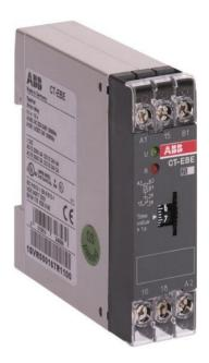
The CT-EBE is a single-function electronic time relay from the CT-E timer range. It provides a flasher (recycling equal times) function with a time range from  $0.1 \, \text{s}$  to  $10 \, \text{s}$ . This time relay operates with a rated control supply voltage of  $110 - 130 \, \text{V}$  AC and has a  $1 \, \text{c/o}$  (SPDT) output rated at  $250 \, \text{V}$  /  $4 \, \text{A}$ .
