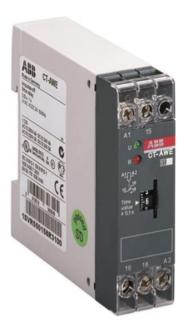
The CT-AWE is a single-function electronic time relay from the CT-E timer range. It provides an impulse-OFF (trailing edge interval) function with a time range from 0.05 s to 1 s. This time relay operates with a rated control supply voltage of 220 - 240 V AC and has a 1 c/o (SPDT) output rated at 250 V / 4 A. A control input works with voltage-related (non-floating) triggering.
