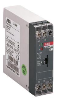
The CT-AWE is a single-function electronic time relay from the CT-E timer range. It provides an impulse-OFF (trailing edge interval) function with a time range from 0.1~s to 10~s. This time relay operates with a rated control supply voltage of 220~-240~V AC and has a 1~c/o (SPDT) output rated at 250~V/4 A. A control input works with voltage-related (non-floating) triggering.
