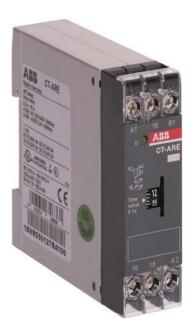
The CT-ARE is a single-function electronic time relay from the CT-E timer range. It provides an OFF-delay (true delay on break) function without auxiliary voltage and with a time range from 0.1 s to 10 s. This time relay operates with a rated control supply voltage of 24 V AC / DC / 220 - 240 V AC and has a 1 c/o (SPDT) output rated at 250 V / 4 A.
