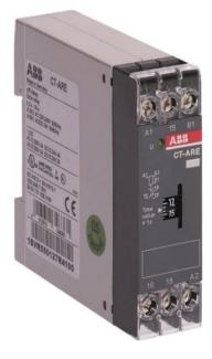
The CT-ARE is a single-function electronic time relay from the CT-E timer range. It provides an OFF-delay (true delay on break) function without auxiliary voltage and with a time range from 0.1 s to 10 s. This time relay operates with a rated control supply voltage of 110 - 130 V AC and has a 1 c/o (SPDT) output rated at 250 V / 4 A.
