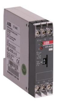
The CT-AHE is a single-function electronic time relay from the CT-E timer range. It provides an OFF-delay (delay on break) function with a time range from 0.1~s to 10~s. This time relay operates with a rated control supply voltage of 24~V AC / DC and has a 1~c/o (SPDT) output rated at 250~V / 4~A. A control input works with voltage-related (non-floating) triggering.
