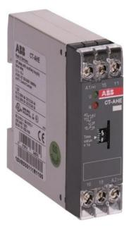
The CT-AHE is a single-function electronic time relay from the CT-E timer range. It provides an OFF-delay (delay on break) function with a time ranges from 0.1 s to 10 s. This time relay operates with a rated control supply voltage of 110 - 130 V AC and has a 1 c/o (SPDT) output rated at 250 V / 4 A. A control input works with voltage-related (non-floating) triggering.
