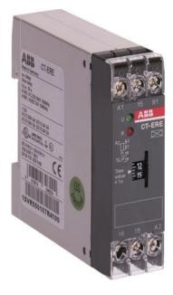
The CT-ERE is a single-function electronic time relay from the CT-E timer range. It provides an ON-delay (delay on make) function with a time range from 0.3 min. to 30 min. This time relay operates with a rated control supply voltage of 110 - 130 V AC and has a 1 c/o (SPDT) output rated at 250 V / 4 A.
