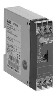
The CT-MKE is a multifunction electronic time relay from the CT-E timer range. It provides 4 timing functions with 2 time ranges from 0.1~s to 300~s. This time relay operates with a rated control supply voltage of 24~-240~V AC / DC and has a solid-state output.
