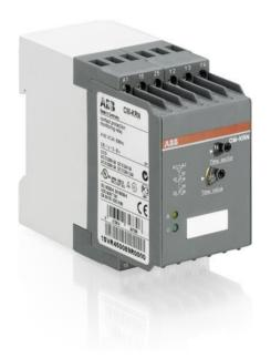
The CM-KRN relay is from the CM contact protection relay range. This protection relay operates with a rated control supply voltage of 24 V AC, has a 2 c/o (SPDT) output with contactst rated at 250 V / 4 A and works according to the open-circuit principle. It acts as two-position switch and protects and reduces load from sensitive control contacts. It can be used with or without latching function. A sealable transparent cover for protection against unauthorized changes is available as accessory.
