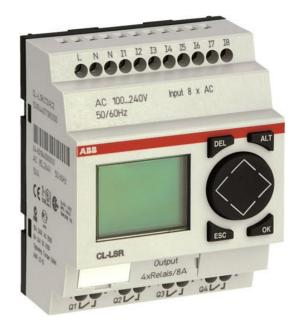
The CL-LSR.C12AC1 is a logic relay from the CL range. It has 8 digital inputs and 4 relay outputs. The logic relay operates with an input voltage of 24 V AC and is equipped with an onboard display and a keypad. 128 rungs with 3 contacts in series plus 1 coil can be programmed. The following functions are available: 16 freely editable display texts, 8 week and 8 year timers, 16 multifunction timing relays, 4 operating hours counters, 16 analog value comparators and threshold value switches
