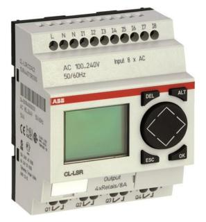
The CL-LSR.C12DC1 is a logic relay from the CL range. It has 8 digital inputs and 4 relay outputs. The logic relay operates with an input voltage of 12 V DC and is equipped with an onboard display and a keypad. 128 rungs with 3 contacts in series plus 1 coil can be programmed. The following functions are available: 16 freely editable display texts, 8 week and 8 year timers, 16 multifunction timing relays, 4 operating hours counters, 16 analog value comparators and threshold value switches
