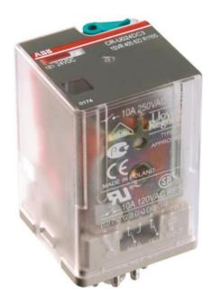
The CR-U048DC3L pluggable interface relay is from the CR-U (universal) relay range. This relay operates with a 48 V DC rated control supply voltage and has 3 c/o (SPDT) output contacts rated at 250 V / 10 A. The relay has an integrated blue test button for manual actuation and locking of the output contacts and an integrated LED. Standard sockets, logic sockets, pluggable function modules, holder and marker are available as accessories.
