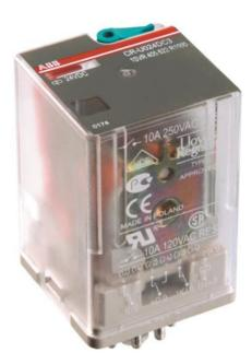
The CR-U110DC2L pluggable interface relay is from the CR-U (universal) relay range. This relay operates with a  $110\ V$  DC rated control supply voltage and has  $2\ c/o$  (SPDT) output contacts rated at  $250\ V$  /  $10\ A$ . The relay has an integrated blue test button for manual actuation and locking of the output contacts and an integrated LED. Standard sockets, logic sockets, pluggable function modules, holder and marker are available as accessories.
