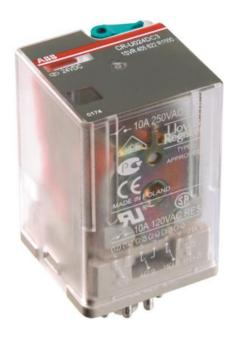
The CR-U110AC2L pluggable interface relay is from the CR-U (universal) relay range. This relay operates with a 110 V AC rated control supply voltage and has 2 c/o (SPDT) output contacts rated at 250 V / 10 A. The relay has an integrated orange test button for manual actuation and locking of the output contacts and an integrated LED. Standard sockets, logic sockets, pluggable function modules, holder and marker are available as accessories.
