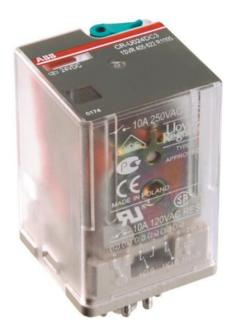
The CR-U024DC2L pluggable interface relay is from the CR-U (universal) relay range. This relay operates with a 24 V DC rated control supply voltage and has 2 c/o (SPDT) output contacts rated at 250 V / 10 A. The relay has an integrated blue test button for manual actuation and locking of the output contacts and an integrated LED. Standard sockets, logic sockets, pluggable function modules, holder and marker are available as accessories.
