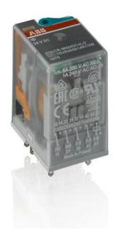
The CR-M048AC3L pluggable interface relay is from the CR-M (miniature) relay range. This relay operates with a 48 V AC rated control supply voltage and has a 3 c/o (SPDT) output with contacts rated at 250 V / 10 A. The relay has an integrated orange test button for manual actuation and locking of the output contacts and an integrated LED. Standard sockets, logic sockets, pluggable function modules, holder and marker are available as accessories.
