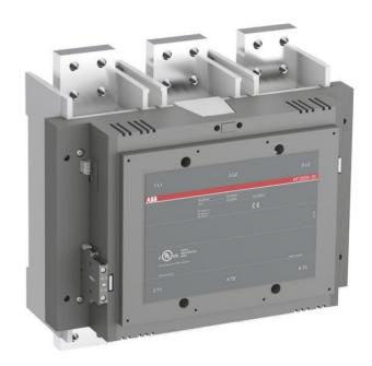
A 3-phase Contactor suitable for various applications such as Isolation, By-pass and Distribution application up to max 1000 V. Operated with wide control voltage range 100-250 V, AC/DC
