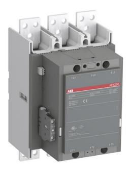
A 3-phase Contactor suitable for various applications such as, Isolation, By-pass and Distribution application up to max 1000 V. Operated with wide control voltage range 250-500 V, AC/DC
