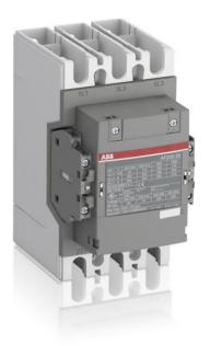
A 3-phase Contactor suitable for various applications such as Motor starting, Isolation, By-pass and Distribution application up to max 1000 V. Operated with wide control voltage range 48-130 V, 50/60 Hz and DC
