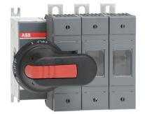
Including terminal bolt kit, a black ON-OFF plastic handle and shaft as standard. The handle is IP65 protected, padlockable in the OFF-position and with door interlock in the ON-position. The shaft is adjustable for a range of installation depths.
