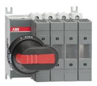
Including terminal bolt kit, a black ON-OFF plastic handle and shaft as standard. The handle is IP65 protected, padlockable in the OFF-position and with door interlock in the ON-position. The shaft is adjustable for a range of installation depths.
