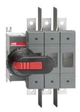
Including terminal bolt kit, a black ON-OFF plastic handle and shaft as standard. The handle is IP65 protected, padlockable in the OFF-position and with door interlock in the ON-position. The shaft is adjustable for a range of installation depths.
