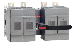
Including terminal bolt kit, a black ON-OFF plastic handle and shaft as standard. The handle is IP65, NEMA 1, 3R, 12 protected, padlockable in the OFF-position and with door interlock in the ON-position. The shaft is adjustable for a range of installation depths. Fuse standards UL 248.
