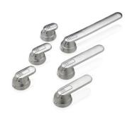
Selector type handle. Indication I-O and ON-OFF. No separate shaft needed. Padlockable with max. 3 padlocks, IP 65, hole distance 36/48 mm, NEMA 1, 3R, 12, red-yellow, OT16...125FT
