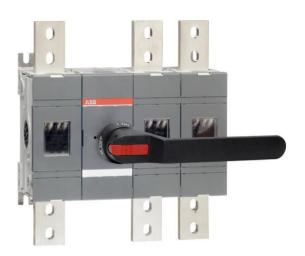
Including a black ON-OFF plastic handle and shaft as standard. The handle is IP65 protected, padlockable in the OFF-position and with door interlock in the ON-position. The shaft is adjustable for a range of installation depths.
