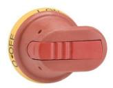
IP65, NEMA 1, 3R, 12, padlockable with three padlocks in OFF-position, door interlock in ON- position. Screw fixing from the back side of the handle. No screws on the front ensures double insulation. The type and the ordering numbers are for one piece, red-yellow.
